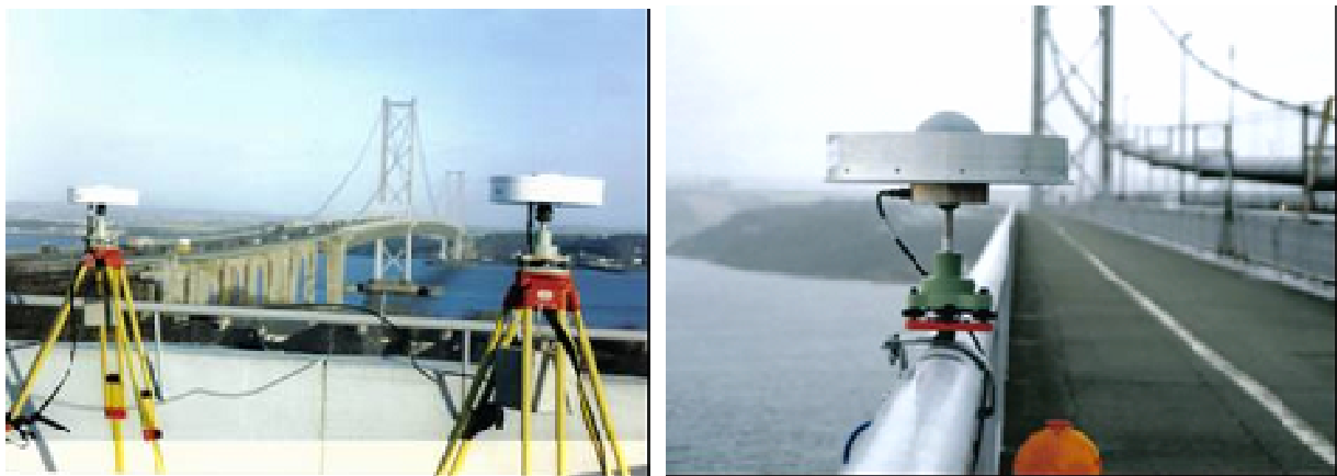
Figure 10. Two GPS reference receivers located adjacent to the Forth road bridge (left). A GPS choke ring antenna attached to the bridge (right).
