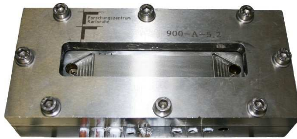
Fig. 4. Electrically powered microstructure device, providing exchangeable micro channel foils and a glass lid for high speed videography
