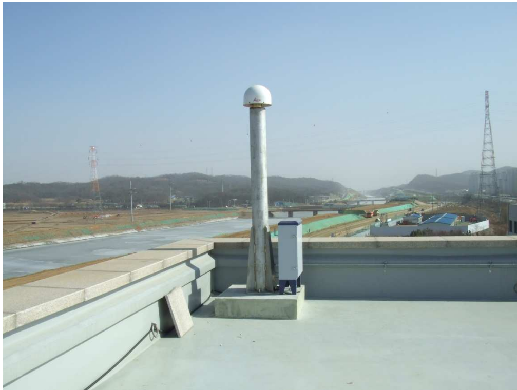
Fig. 2. One of the GLONASS and GPS Reference station on the roof top of NAH office
