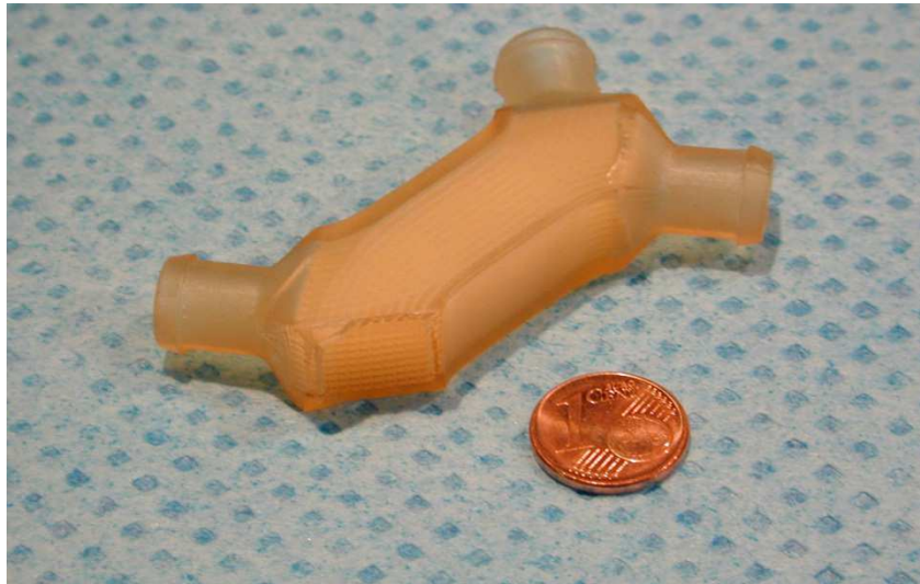
Fig. 2: polymer counterflow microstructure heat exchanger made by micro stereo lithography Devices like this one are relatively easy to manufacture and useful either for fast experimental analysis of special design variations or for visualization of device design
