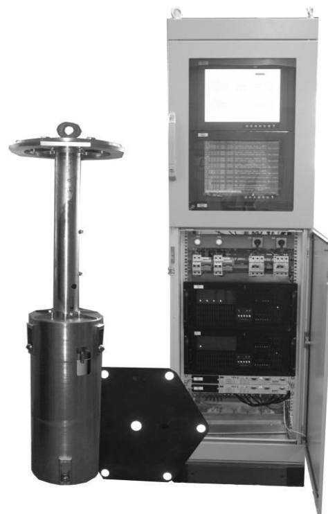
Fig. 7. System SAKHALIN: optical measuring and electronic units.
