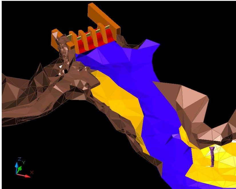
Figure 9: Model of the existing weir
