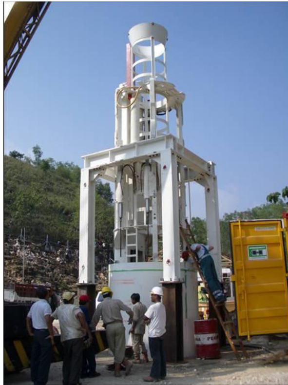
Figure 6: Vertical drilling machine VSM 2500
